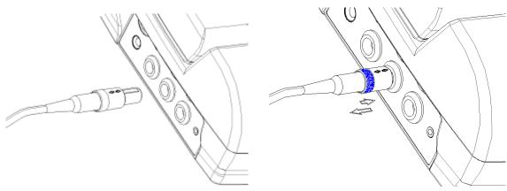
Figure 6-1 Connecting the transducer
