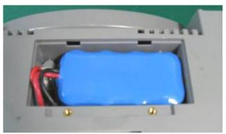
6) Shut the battery compartment cover and fix the screws.
