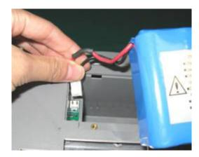
5) Put the battery and the cables into the battery compartment.
