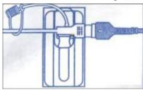
Figure 8-5 Secure the adhesive pad to mother
