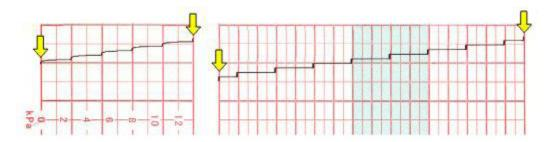
If the monitor does not print the baseline, switch on the Print Self-Check and then restart the monitor.
