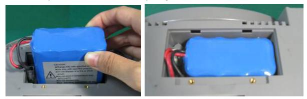
5) Shut the battery compartment cover and fix the screws.
