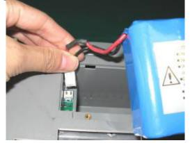
4) Put the battery and the cables into the battery compartment.
